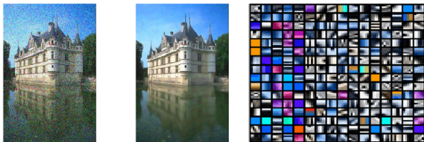
Figure: Left: noisy input; middle: denoised; right: learned patch dictionary.
